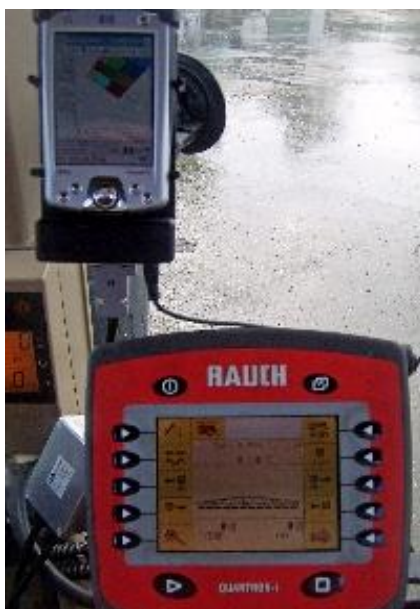
Farm Works Site Mate VRA Solution connected to the Rauch Quantron I
